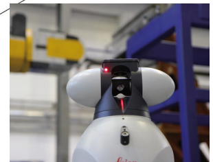
Inbuilt RCMT measurement system / laser tracker for contactless position measurements and evaluation of the machine tool static errors
