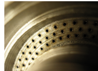
Holes by laser drilling
