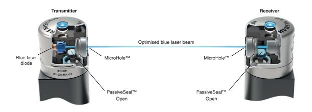
While conventional laser tool setting systems feature a red laser beam, NC4+ Blue is the industry's first blue laser tool setter. Blue lasers have a shorter wavelength, resulting in improved diffraction effects and optimised laser beam geometry.
