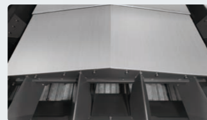
Enlarged chip ducts for smooth chip disposal
