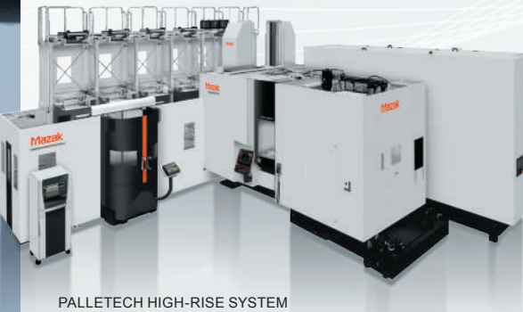
PALLETECH HIGH-RISE SYSTEM (3-level stocker with 18 pallets and one loading station)
