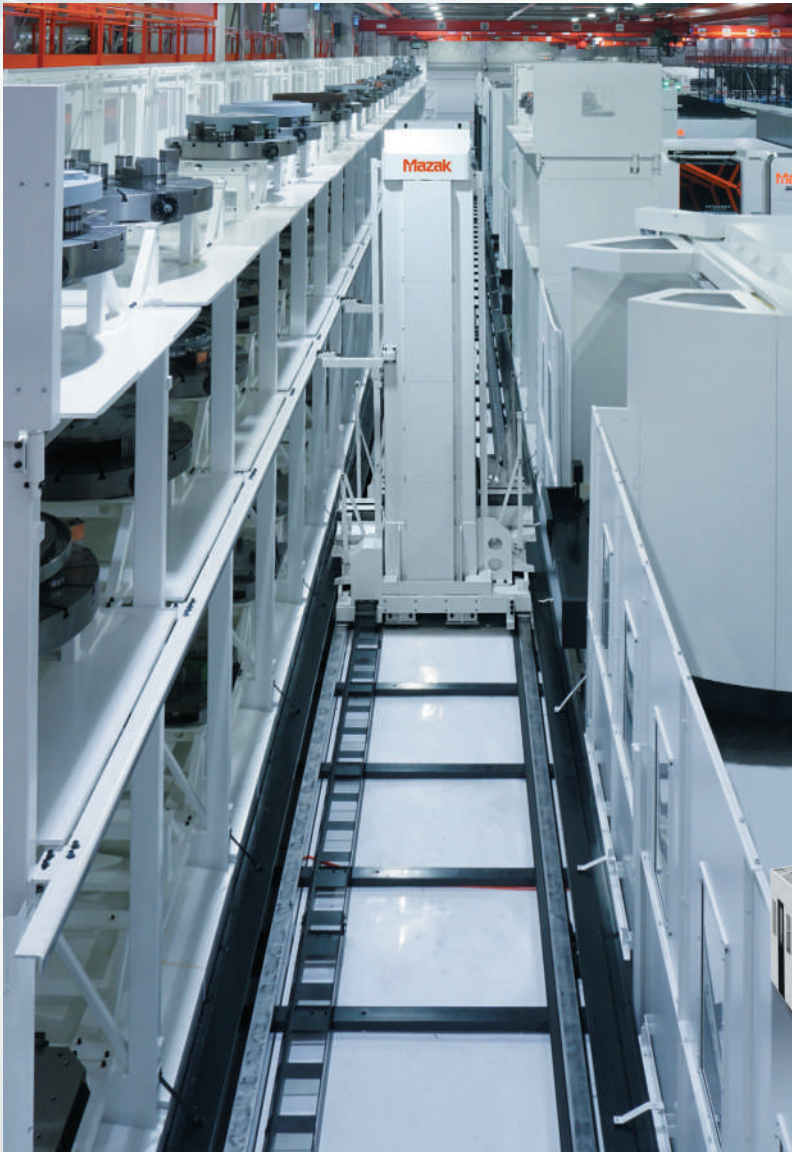
PALLETECH HIGH-RISE SYSTEM (3-level stocker with 18 pallets and one loading station)
