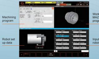
Workpiece display from MAZATROL machining program
